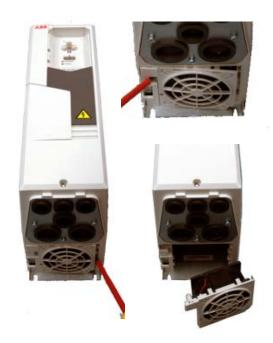
d. Check that the fans blowing direction is inside the unit and install the new fan in reverse order to above. Ensure the fan operation when the drive is powered up
