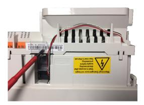
2. Unlock the wires from the right and take slowly the fan out by pulling the wires.
