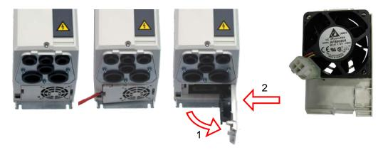
d. Check that the fans blowing direction is inside the unit and install the new fan unit simply by pushing it to its place.
