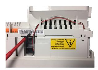
2. Unlock the wires from the right and take slowly the fan out by pulling the wires.
