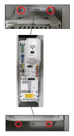
Place collar around drive. Using a T20 bit, secure the drive using the six (6) M4x20 screws that were removed earlier.
