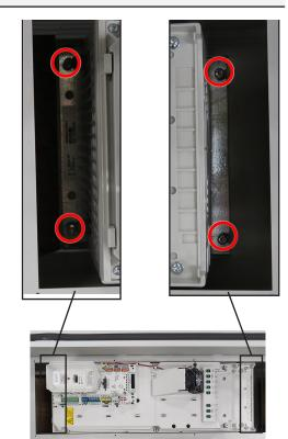
8 Carefully push the drive up, lift the drive off the screws and out of enclosure.
