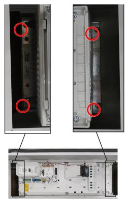
Place collar around drive. Using a T20 bit, secure the drive using the M4x20 screws that were removed earlier.
