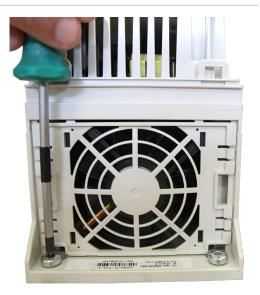
Remove two (2) grommets from the tray to access mounting screws.
