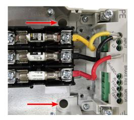
13 Secure the mounting plate using the four (4) M4x8 screws that were removed earlier.
