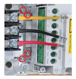
7 Using a T30 bit, loosen the two (2) bottom M5 screws securing the drive, four (4) turns of the screw.
