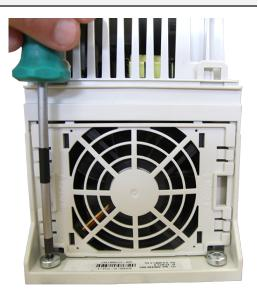
12 Using a T30 bit, replace the two (2) M5 screws that were removed
