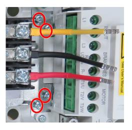
**14** Secure the ground wire to the drive.
