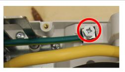
Connect the input wires (from fuse block) to the Input Terminals of the drive.
