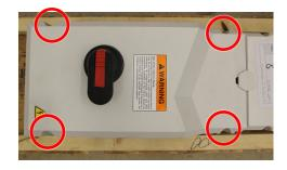
**3 UL Type 1:** Using a T20 bit, loosen one (1) M4x16 screws securing the drive cover and remove cover.
