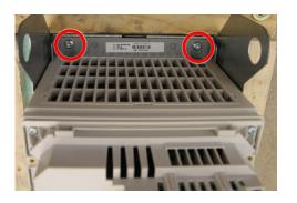
**9** Remove two (2) grommets from the tray to access mounting screws.
