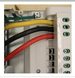
**R3 Frame:** Using a T20 bit, loosen and remove four (4) K40x12 screws. Remove conduit assembly.
