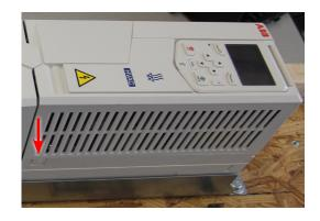
Place enclosure cover in place and secure using two (2) M4x16 screws that were removed earlier.
