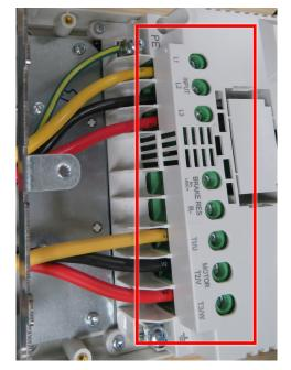
**16** Connect the input wires (from fuse block) to the Input Terminals of the drive.
