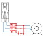
Figure 12: A *dV/dt* filter reduces the rate of rise of the PWM pulse and controls voltage overshoot.
