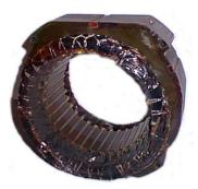
Figure 1: A motor stator with over-heated insulation.
