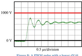
Figure 8: A PWM pulse with a lower *dV/dt* value creates a lower voltage overshoot.
