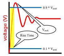
Figure 4: When a voltage pulse reaches a motor, it overshoots and oscillates.
